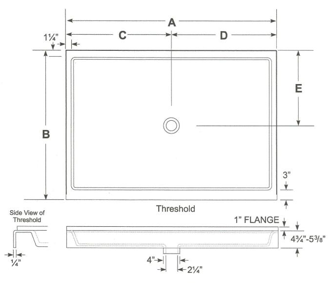
Single threshold center drain shower pans have a 1" flange on three sides for *AmeriWall* 3 wall shower enclosure applications and come with a self-caulking wedge-lock drain and strainer. The white color of the pans is a very close match to AmeriWall. The pans are molded from a single piece of durable, stain and fungus resistant composite material and feature a non-slip surface that doesn't interfere with the flow of water.
