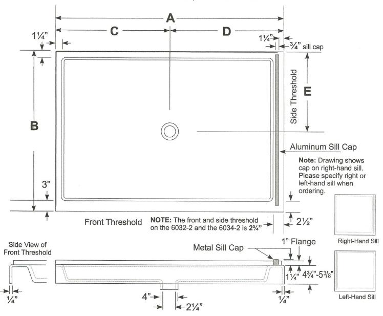
Double threshold center drain shower pans have a 1" flange on two sides for *AmeriWall* 2-wall shower enclosure applications and come with a self-caulking, wedge-lock drain and strainer. The sill adjacent to the left or right side of the threshold has an aluminum cap to receive a glass wall.
